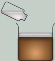
Pastes that have dried out and cannot be dispensed should not be reconstituted. Dedicated binder system thinners with specific properties are used to thin pastes in production to the correct work viscosity. Any attempt to reconstitute a product is unlikely to result in a paste that will function effectively.
