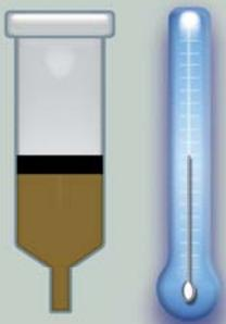
Braze and soft solder pastes should not be stored below 5°C or above 25°C. The ideal storage temperature for pastes is between 10 and 15°C.
